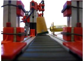
With **IPTS-3** Software, there is a suite of 6 different programs or projects. Each program or project when loaded into the PLC will immediately present a different fault scenario which will need to be investigated. The challenge is to identify the problem & to suggest how it could be resolved. These faults demand a more thorough understanding of how the PLC operates & are more challenging.
